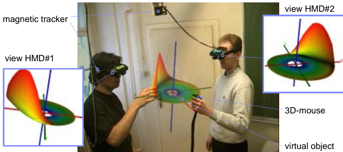
Figure 7: Two users investigating the Rössler-attractor in the Studierstube setup. Due to the direct correspondence of positions in real world and the augmentation, simple interactions, e.g. pointing are possible and enrich communication.
