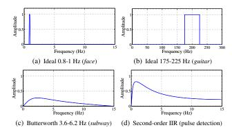
**Figure 9:** Temporal filters used in the paper. The ideal filters (a) and (b) are implemented using DCT. The Butterworth filter (c) is used to convert a user-specified frequency band to a second-order IIR structure and is used in our real-time application. The second-order IIR filter (d) also allows user input. These second-order filters have a broader passband than an ideal filter.
