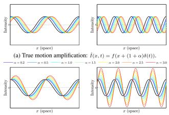
(b) Motion amplification via temporal filtering:  $\tilde{I}(x,t) = I(x,t) + \alpha B(x,t)$ .
