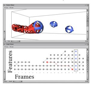
**Figure 11:** One step during feature tracking. A path is shown with its prediction, and three candidates in the next time step [52].
