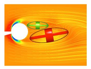
**Figure 18:** *Vortices behind a tapered cylinder. The colour of the ellipsoids represents the rotational direction* [28].
