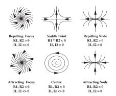
**Figure 1:** Vector field topology: critical points classified by the eigenvalues of the Jacobian [6].
