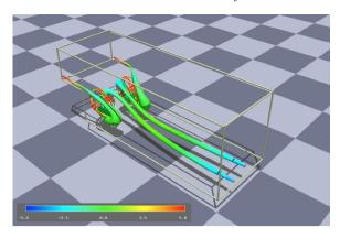
Figure 15: Visualisation with streamtubes of the recirculation in the backward-facing-step data set [55].
