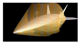
**Figure 5:** A shockwave around an aircraft (H.-G. Pagendarm).
