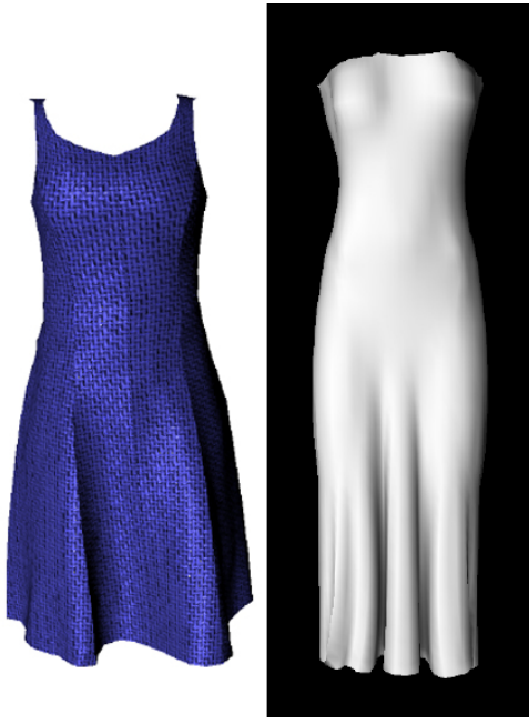
Figure 10: left: A dress rendered with a spatially varying BRDF consisting of one lobe (from [Daubert et al. 2001]). right: A folded dress consisting of 3120 vertices rendered with the help of binary visibility maps (reprinted from [Ganster et al. 2002]).
