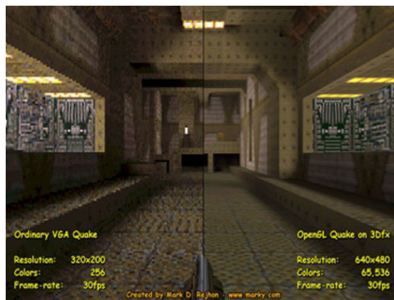
Figure 4: Standard Quake vs Quake using bilinear texture filtering.
