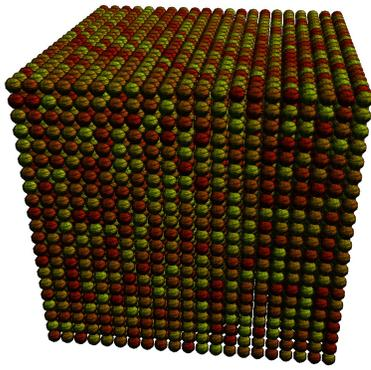
**Figure 8:** Screenshot of our worst case test setup designed to cause a high load on the graphics pipeline: the camera slowly rotates around this grid of spheres which thus remains inside the view frustum at all times.
