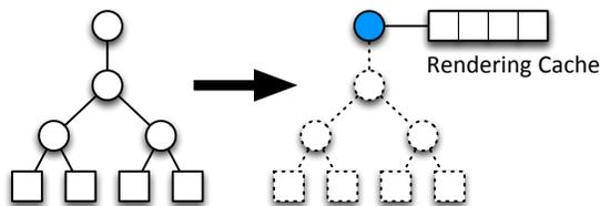
**Figure 1:** A rendering cache captures all rendering instructions in a subgraph and takes over its rendering responsibilities.
