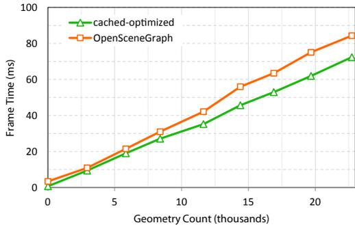
**Figure 12:** Frame times for the static scenes with varying number of geometries in our system with render caches (state sorting and redundancy removal enabled) and in *OpenSceneGraph* (single-threaded).
