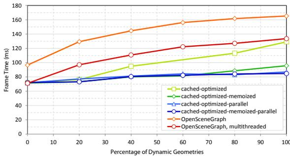
**Figure 15:** Frame times in a scene with a depth complexity of 8 transformations. The scene is structured as an octree with additional dynamic transformation nodes at each level, as shown in Figure 14.
