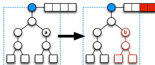
**Figure 4:** An in-place update of a rendering cache due to a modification of an attribute (affected scene graph parts and rendering cache parts shown in red).
