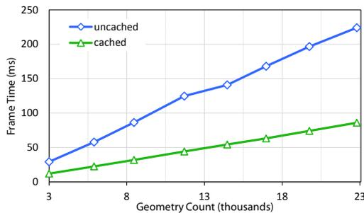
**Figure 9:** Comparison of frame-times for our reference implementation with the proposed caching mechanism in our static scene. While the total scene complexity (number of primitives) is constant the number of geometries (equivalent to draw calls) varies to show the overhead due to the traversal of the scene graphs.
