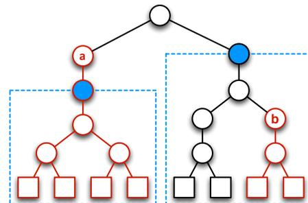
**Figure 3:** Modifying some attributes (*a* and *b*) requires the update of rendering caches (blue nodes) that capture on them (affected scene graph parts are shown in red).
