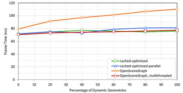
**Figure 13:** Frame times in scenes with varying percentage of moving objects. Transformation matrices are updated each frame – these updates require additional CPU processing due to matrix multiplication but also involve the GPU for resource updates.
