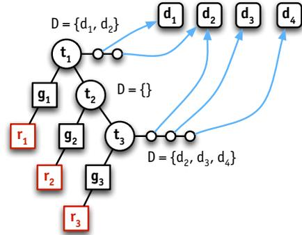
**Figure 6:** A small scene graph with transformation nodes as value sources ( $t_i$ ), a number of dependencies for these value sources ( $d_j$ ), a number of geometries ( $g_k$ ), and a number of dependent resources ( $r_l$ ).
