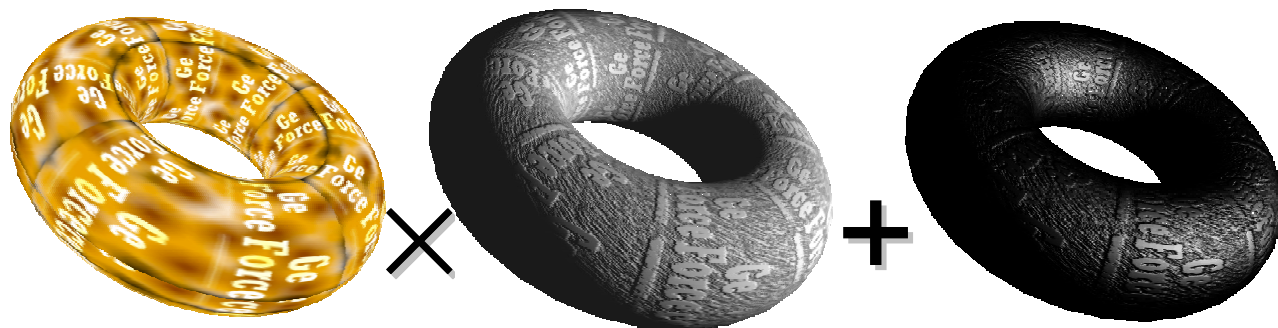
Figure 12. Torus rendered with the new bump mapping technique. Specular, diffuse, and ambient lighting contributions are all present along with a surface decal texture.
