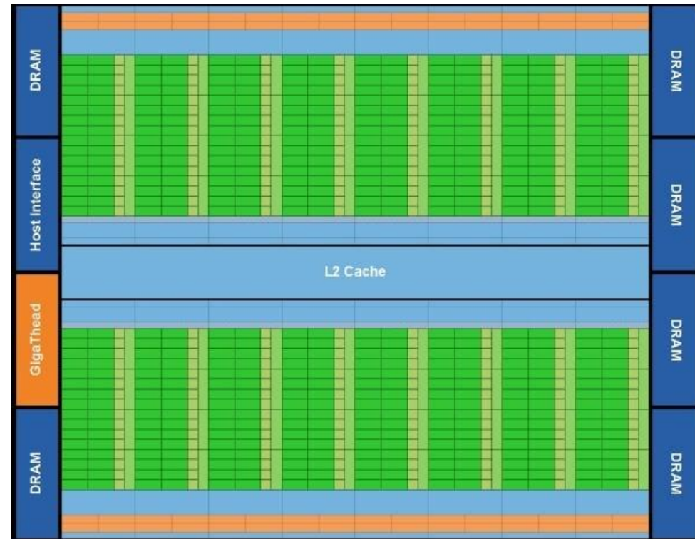
Fermi's 16 SM are positioned around a common L2 cache. Each SM is a vertical rectangular strip that contain an orange portion (scheduler and dispatch), a green portion (execution units), and light blue portions (register file and L1 cache).
