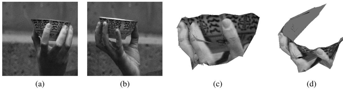
**Figure 7.6** 3D teacup model reconstructed from a 240-frame video sequence (Tomasi and Kanade 1992) © 1992 Springer: (a) first frame of video; (b) last frame of video; (c) side view of 3D model; (d) top view of 3D model.
