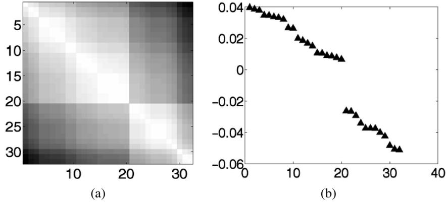
**Figure 5.20** Sample weight table and its second smallest eigenvector (Shi and Malik 2000) © 2000 IEEE: (a) sample  $32 \times 32$  weight matrix  $\mathbf{W}$ ; (b) eigenvector corresponding to the second smallest eigenvalue of the generalized eigenvalue problem  $(\mathbf{D} - \mathbf{W})\mathbf{y} = \lambda\mathbf{D}\mathbf{y}$ .
