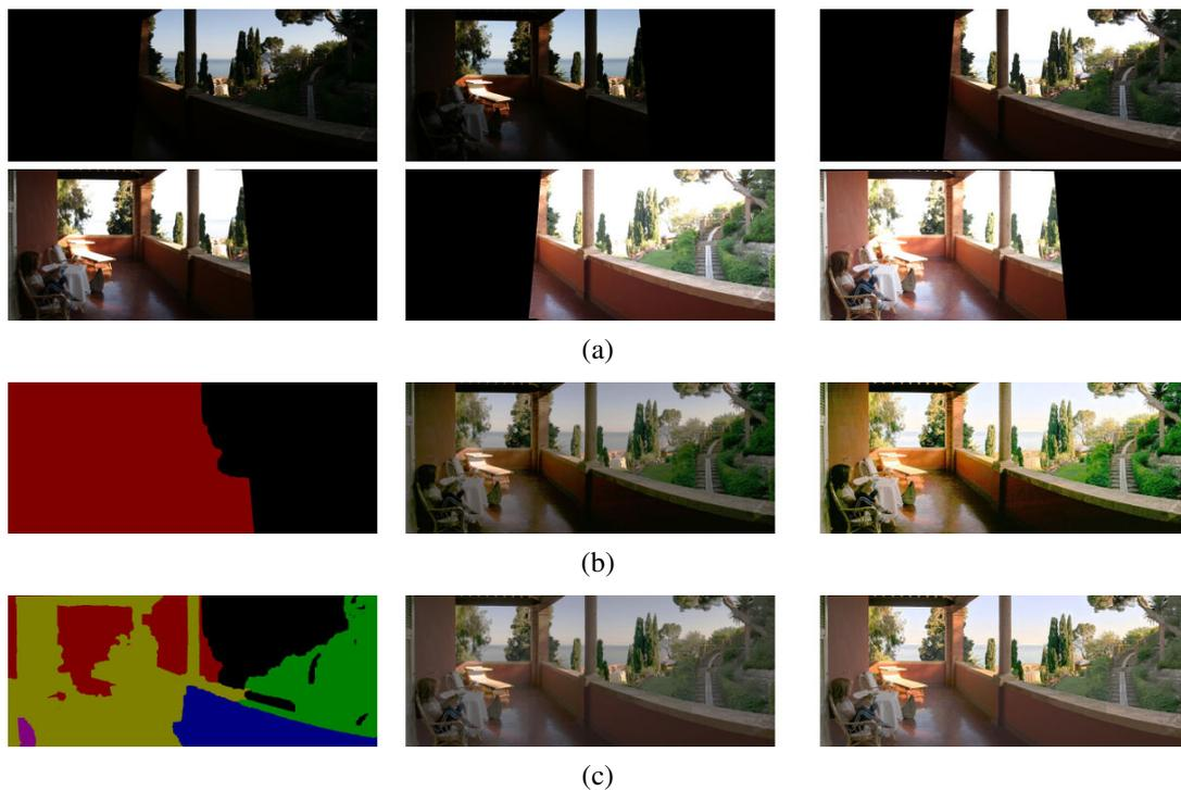
**Figure 10.17** HDR merging with large amounts of motion (Eden, Uyttendaele, and Szeliski 2006) © 2006 IEEE: (a) registered bracketed input images; (b) results after the first pass of image selection: reference labels, image, and tone-mapped image; (c) results after the second pass of image selection: final labels, compressed HDR image, and tone-mapped image
