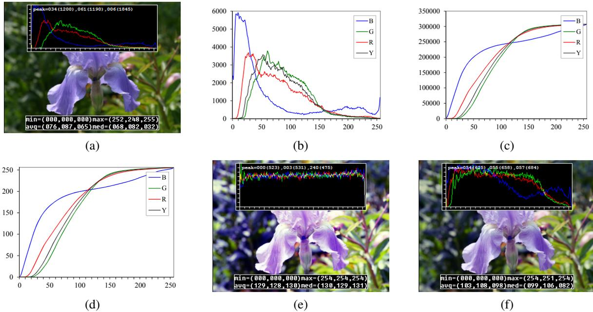
**Figure 3.7** Histogram analysis and equalization: (a) original image (b) color channel and intensity (luminance) histograms; (c) cumulative distribution functions; (d) equalization (transfer) functions; (e) full histogram equalization; (f) partial histogram equalization.
