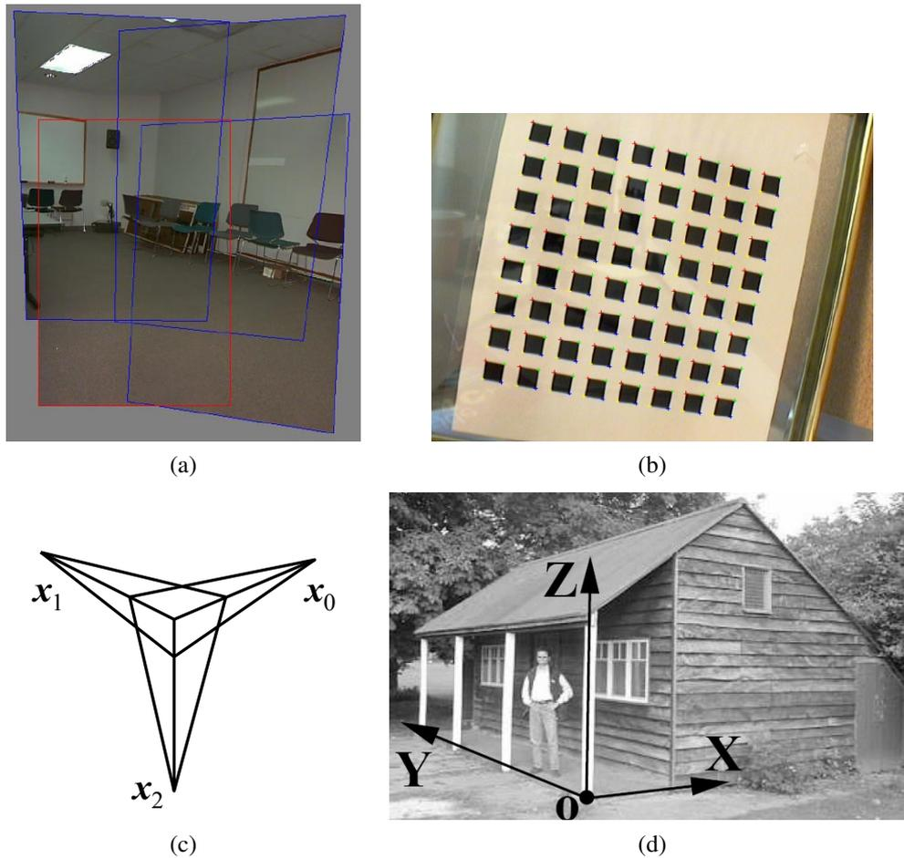
**Figure 6.1** Geometric alignment and calibration: (a) geometric alignment of 2D images for stitching (Szeliski and Shum 1997) © 1997 ACM; (b) a two-dimensional calibration target (Zhang 2000) © 2000 IEEE; (c) calibration from vanishing points; (d) scene with easy-to-find lines and vanishing directions (Criminisi, Reid, and Zisserman 2000) © 2000 Springer.
