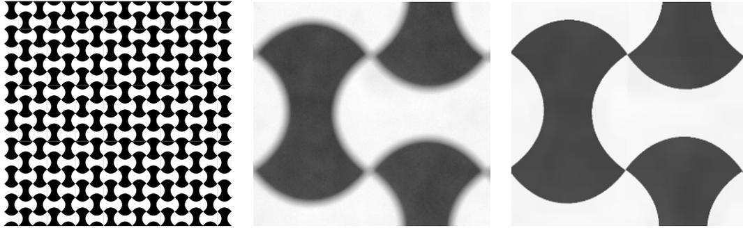
**Figure 10.7** Calibration pattern with edges equally distributed at all orientations that can be used for PSF and radial distortion estimation (Joshi, Szeliski, and Kriegman 2008) © 2008 IEEE. A portion of an actual sensed image is shown in the middle and a close-up of the ideal pattern is on the right.
