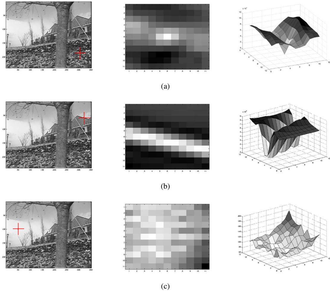
**Figure 8.4** SSD surfaces corresponding to three locations (red crosses) in an image: (a) highly textured area, strong minimum, low uncertainty; (b) strong edge, aperture problem, high uncertainty in one direction; (c) weak texture, no clear minimum, large uncertainty.
