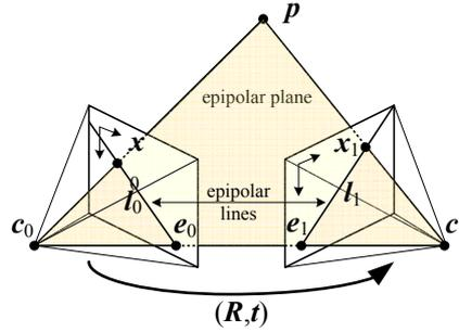
**Figure 7.3** Epipolar geometry: The vectors  $\mathbf{t} = \mathbf{c}_1 - \mathbf{c}_0$ ,  $\mathbf{p} - \mathbf{c}_0$  and  $\mathbf{p} - \mathbf{c}_1$  are co-planar and define the basic epipolar constraint expressed in terms of the pixel measurements  $\mathbf{x}_0$  and  $\mathbf{x}_1$ .
