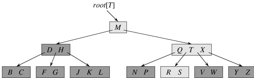
**Figure 18.1** A B-tree whose keys are the consonants of English. An internal node  $x$  containing  $n[x]$  keys has  $n[x] + 1$  children. All leaves are at the same depth in the tree. The lightly shaded nodes are examined in a search for the letter  $R$ .
