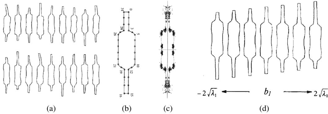
**Figure 5.4** Point distribution model for a set of resistors (Cootes, Cooper, Taylor *et al.* 1995) © 1995 Elsevier: (a) set of input resistor shapes; (b) assignment of control points to the boundary; (c) distribution (scatter plot) of point locations; (d) first (largest) mode of variation in the ensemble shapes.
