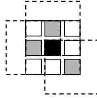
**Figure 11.8** Shiftable window (Scharstein and Szeliski 2002) © 2002 Springer. The effect of trying all  $3 \times 3$  shifted windows around the black pixel is the same as taking the minimum matching score across all *centered* (non-shifted) windows in the same neighborhood. (For clarity, only three of the neighboring shifted windows are shown here.)
