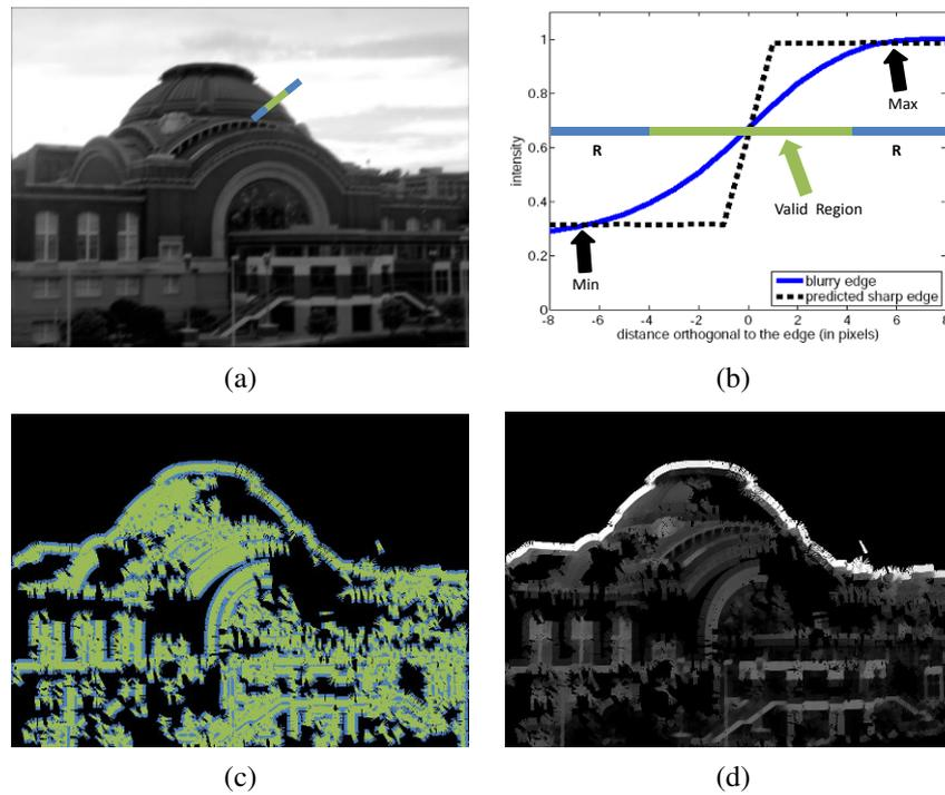
**Figure 10.9** Estimating the PSF without using a calibration pattern (Joshi, Szeliski, and Kriegman 2008) © 2008 IEEE: (a) Input image with blue cross-section (profile) location, (b) Profile of sensed and predicted step edges, (c–d) Locations and values of the predicted colors near the edge locations.
