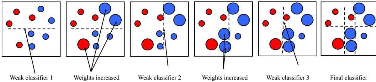
**Figure 14.7** Schematic illustration of boosting, courtesy of Svetlana Lazebnik, after original illustrations from Paul Viola and David Lowe. After each weak classifier (decision stump or hyperplane) is selected, data points that are erroneously classified have their weights increased. The final classifier is a linear combination of the simple weak classifiers.
