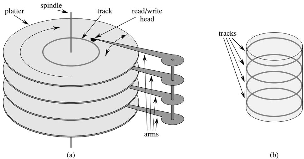
**Figure 18.2** (a) A typical disk drive. It is composed of several platters that rotate around a spindle. Each platter is read and written with a head at the end of an arm. The arms are ganged together so that they move their heads in unison. Here, the arms rotate around a common pivot axis. A track is the surface that passes beneath the read/write head when it is stationary. (b) A cylinder consists of a set of covertical tracks.
