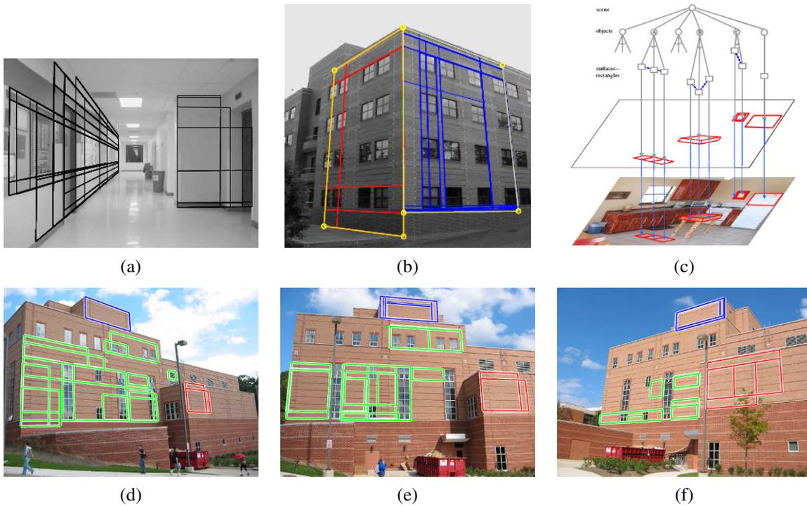
**Figure 4.47** Rectangle detection: (a) indoor corridor and (b) building exterior with grouped facades (Košecká and Zhang 2005) © 2005 Elsevier; (c) grammar-based recognition (Han and Zhu 2005) © 2005 IEEE; (d–f) rectangle matching using a plane sweep algorithm (Mičušík, Wildenauer, and Košecká 2008) © 2008 IEEE.
