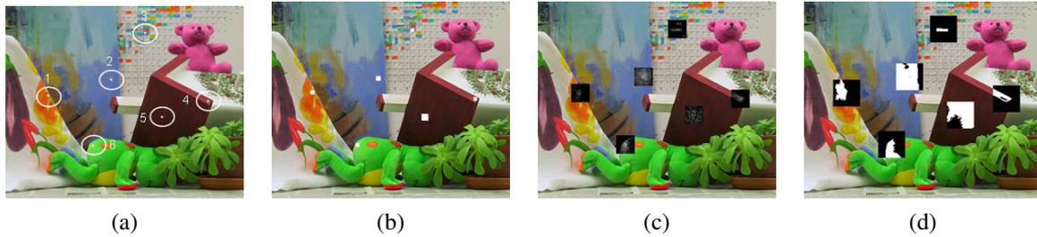
**Figure 11.9** Aggregation window sizes and weights adapted to image content (Tombari, Mattoccia, Di Stefano *et al.* 2008) © 2008 IEEE: (a) original image with selected evaluation points; (b) variable windows (Veksler 2003); (c) adaptive weights (Yoon and Kweon 2006); (d) segmentation-based (Tombari, Mattoccia, and Di Stefano 2007). Notice how the adaptive weights and segmentation-based techniques adapt their support to similarly colored pixels.
