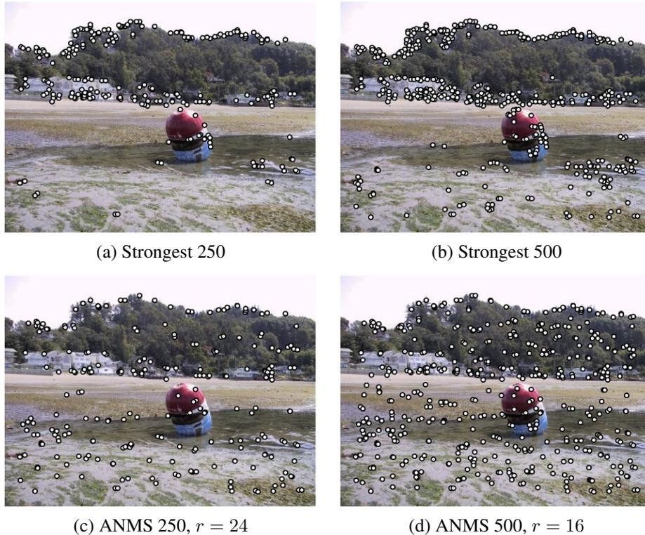
**Figure 4.9** Adaptive non-maximal suppression (ANMS) (Brown, Szeliski, and Winder 2005) © 2005 IEEE: The upper two images show the strongest 250 and 500 interest points, while the lower two images show the interest points selected with adaptive non-maximal suppression, along with the corresponding suppression radius  $r$ . Note how the latter features have a much more uniform spatial distribution across the image.
