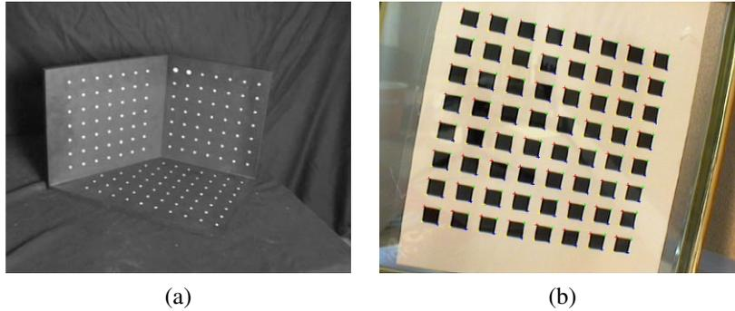
**Figure 6.8** Calibration patterns: (a) a three-dimensional target (Quan and Lan 1999) © 1999 IEEE; (b) a two-dimensional target (Zhang 2000) © 2000 IEEE. Note that radial distortion needs to be removed from such images before the feature points can be used for calibration.
