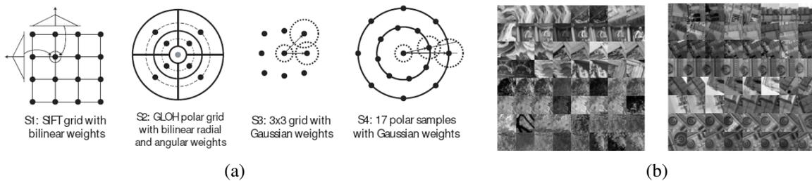
**Figure 4.20** Spatial summation blocks for SIFT, GLOH, and some newly developed feature descriptors (Winder and Brown 2007) © 2007 IEEE: (a) The parameters for the new features, e.g., their Gaussian weights, are learned from a training database of (b) matched real-world image patches obtained from robust structure from motion applied to Internet photo collections (Hua, Brown, and Winder 2007).
