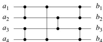
**Figure 27.6** A sorting network for sorting 4 numbers.
