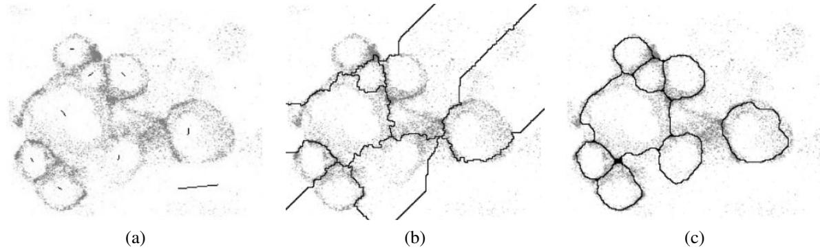
**Figure 5.13** Locally constrained watershed segmentation (Beare 2006) © 2006 IEEE: (a) original confocal microscopy image with marked seeds (line segments); (b) standard watershed segmentation; (c) locally constrained watershed segmentation.
