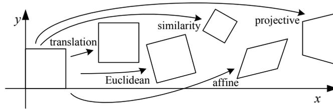
**Figure 6.2** Basic set of 2D planar transformations
