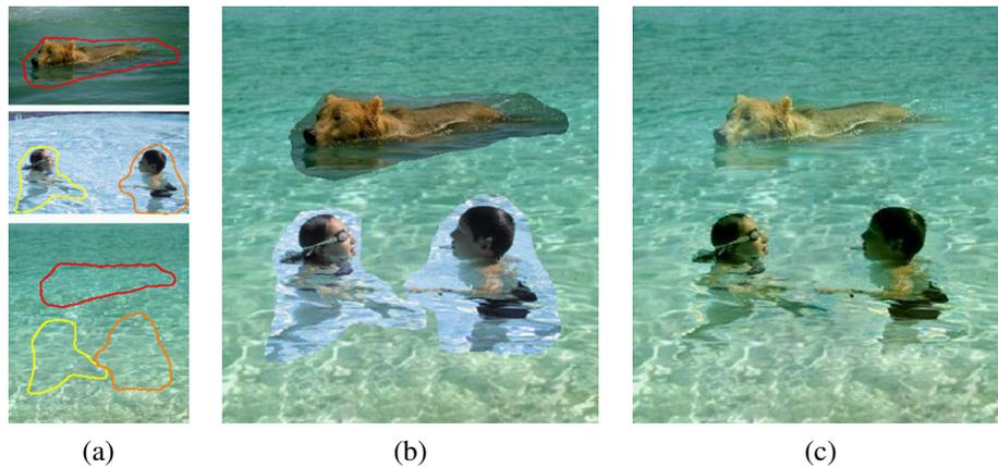
**Figure 9.18** Poisson image editing (Pérez, Gangnet, and Blake 2003) © 2003 ACM: (a) The dog and the two children are chosen as source images to be pasted into the destination swimming pool. (b) Simple pasting fails to match the colors at the boundaries, whereas (c) Poisson image blending masks these differences.
