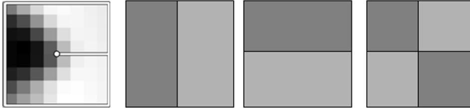
**Figure 4.26** The three Haar wavelet coefficients used for hashing the MOPS descriptor devised by Brown, Szeliski, and Winder (2005) are computed by summing each  $8 \times 8$  normalized patch over the light and dark gray regions and taking their difference.
