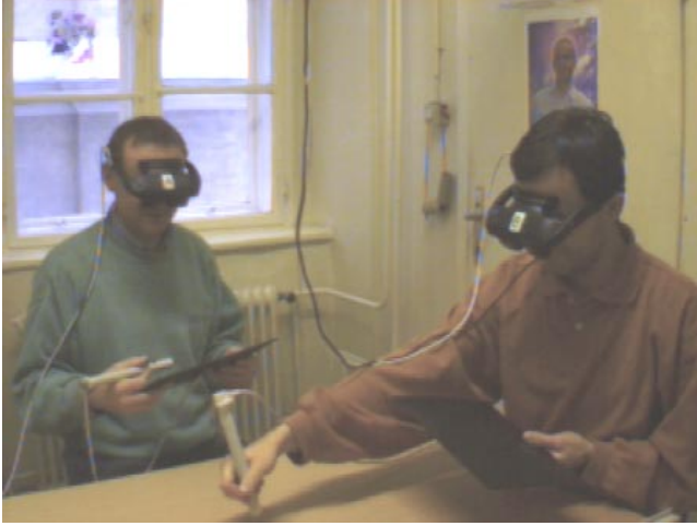
Figure 2. A view onto the hardware environment visible to the players. Each player wears a see-through head-mounted display and interacts with a Personal Interaction Panel.
