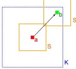
Figure 5: Schematic of the non-local means algorithm for denoising introduced by [Buades et al. 2005].
