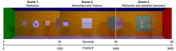
Figure 6: This figure shows the test sequence along the time-line with an image example for each scene. Scene 1 shows two rotating objects with reflective surfaces, each one with a different magnitude of specularity. Scene 2 features a scaling and rotating cube with a detailed diffuse texture. The last scene features a rotating transparent cube.
