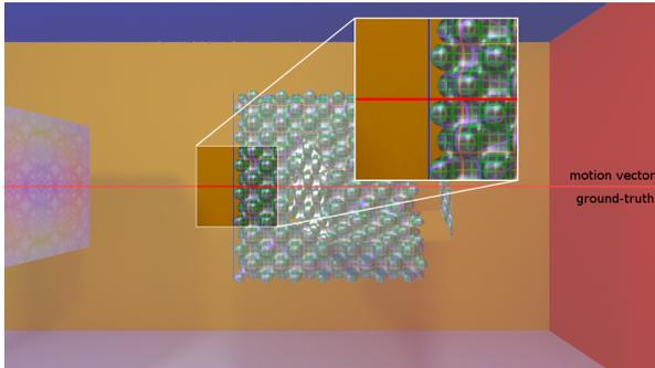
Figure 10: Non-linear motion poses a problem for our approach, since the linear motion vectors can not compensate for such movement.
