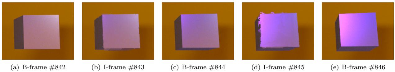
Figure 14: Sequence produced with our proposed technique (brute-force variant). ‘Tearing’ artifacts appear due to rapid color change across a major part of the surface. One can also observe the ghosting in Subfigure (b) as a result of the bottom side of the cube, which was not visible in the previous frame.
