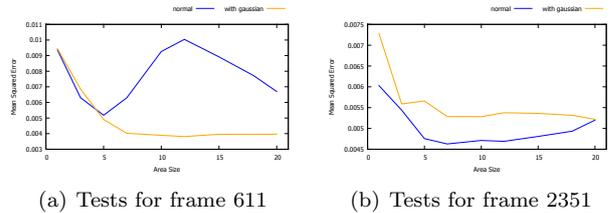
Figure 7: Tests for the size of the similarity area to use in the testing sequence. The blue line depicts the mean squared errors without a Gaussian kernel and the orange line shows a weighting of the area with the kernel.
