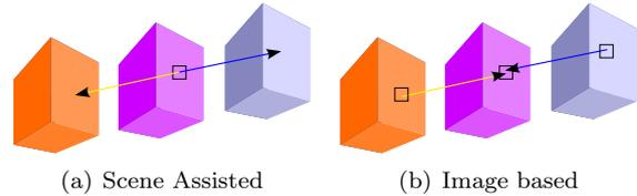
Figure 2: Difference in the data usage of two methods proposed by [Yang et al. 2011]. The scene-assisted approach requires a rendering of the desired frame, whereas the image-based approach does not. In each case the purple cube represents the unknown shading information, the orange one represents the shading from the previous frame and the blue depicts the shading information of the upcoming frame.
