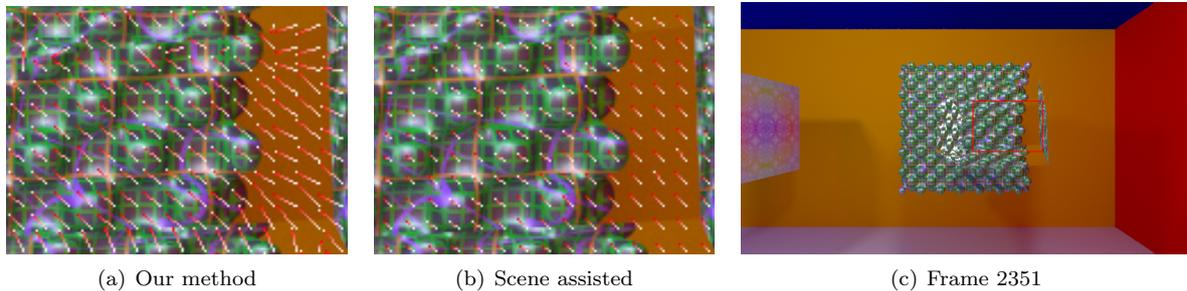
Figure 11: Comparison of the motion vectors generated with our method (left figure) and with the approach by [Yang et al. 2011] (middle figure). Apart from the different length of the motion vectors, one can also notice a different alignment of the motion vectors from our method compared to the one of [Yang et al. 2011]. The motion vectors point from the white towards the red. The right figure shows the part of frame 2351 from our test sequence that is used for this comparison.
