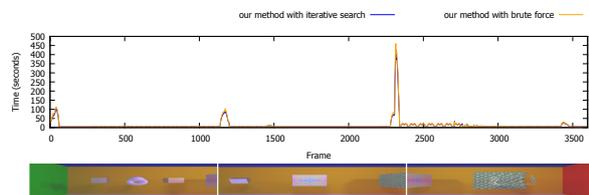
Figure 9: This figure shows the times to generate each frame in seconds on an Intel Core i7-4770K CPU with four 3.50GHz cores. The biggest neighborhood area size for our test sequence is 67.
