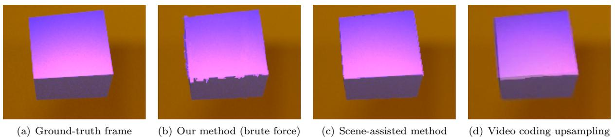
Figure 13: Glass cube in frame 611 of the test sequence with various upsampling techniques. Our method produces a ‘tearing’ artifact due to a flash-like color change on the surface. Upsampling via video coding uses a heuristic in such a case and the scene-assisted method of [Yang et al. 2011] is not affected by such a color change.
