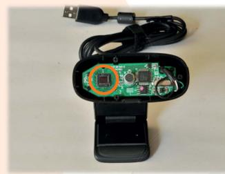
Lens and infrared filter removed
