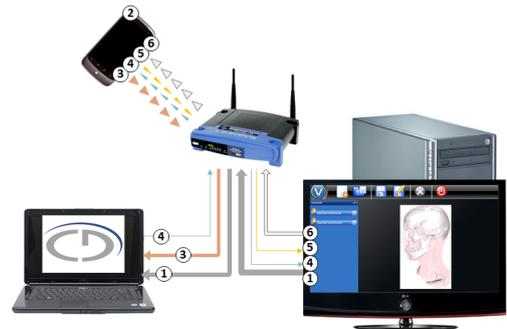
**Figure 5: Prototype of our augmented visualization system. Lines with the same color represent the same data flow. Line width indicates the relative bandwidth need.**
