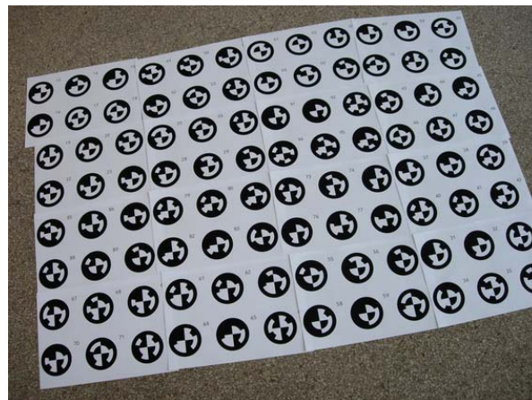
Fig. 1: 96 calibration markers arranged in a 4 by 4 layout on the floor (Irschara et al. 2007)
