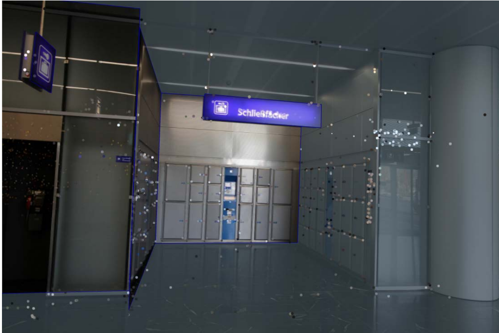
Fig. 2: Point-cloud in a reconstructed 3D environment based on photos
