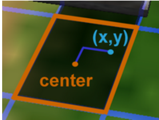
Figure 3.6: An undersampled shadow map texel in screen-space: We define the confidence in the shadowing result at a given fragment at position (x, y) as 1 - \max(|x - center_x|, |y - center_y|) * 2 .
