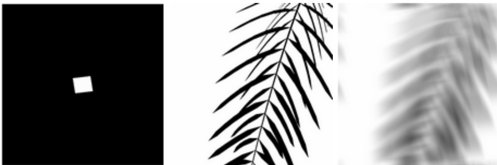
Figure 2.20: The light source image (left), the blocker image (middle) and the convolved result (right). Image courtesy of [SS98].
