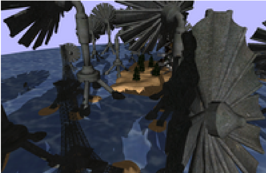
Figure 3.1: Pixel-correct shadow maps as a result of using a shadow map (size 1024^2 ) with shadow test confidence together with a history buffer. Note that projection and perspective aliasing are completely removed.
