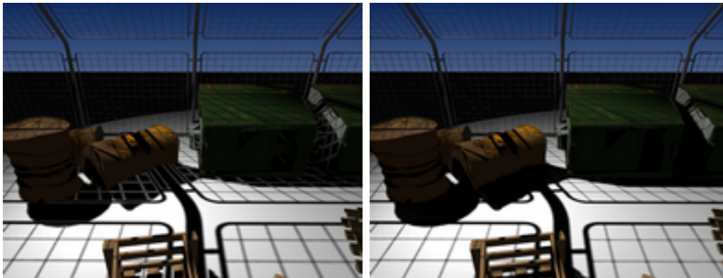
Figure 2.8: Variance shadow maps (left) in contrast to convolution shadow maps (right) suffer from light leaks. Image courtesy of [AMB + 07].
