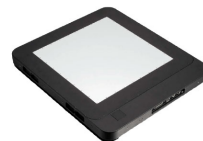
a-Si Flatpanel detector Pixel: 1024^2 Pitch: 400 \mu\text{m}
