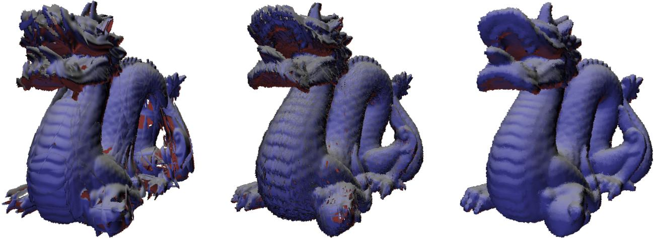
Figure 1: Impostors of the dragon model. Left: traditional billboard cloud with 31 rectangles and 1.76 MB required texture memory. Middle: traditional billboard cloud with 186 rectangles and 11MB required texture memory. Right: displacement mapped billboard cloud with 31 boxes and 10.3 MB required textured memory.
