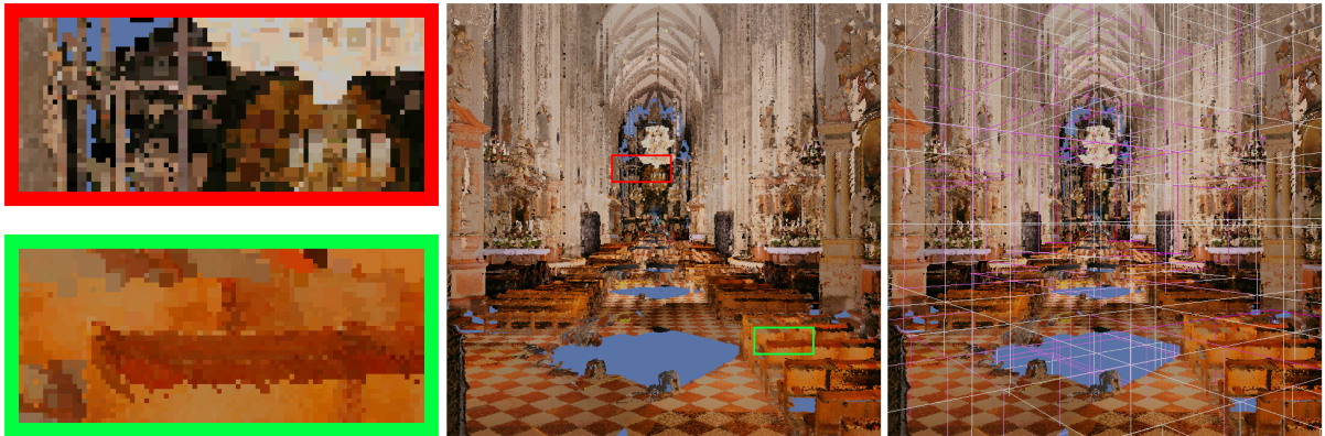
Figure 9: Screenshots of the walkthrough in the cathedral model. The zoomed parts of the middle image show that the point sizes are similar for the far away and for the nearby regions, proving that the LOD selection works well. The middle image was rendered with 9,890,458 points in 308 cells, and loading was completed. In the right image, the magenta bounding boxes indicate that some children of these cells were not rendered because the projected sizes of their bounding boxes were too small.
