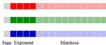
Figure 11: Bit breakdown of the OpenEXR Half encoding.
