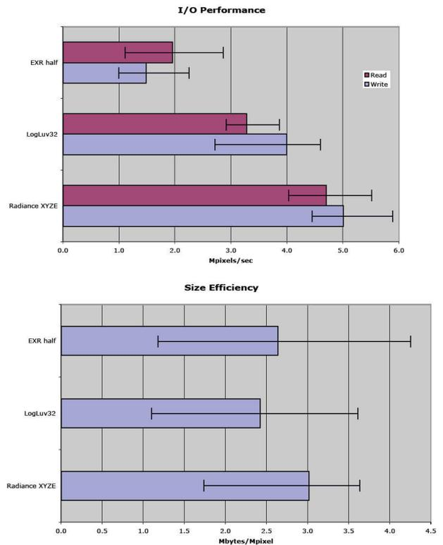
Figure 21: I/O performance and file size comparison. The lines show the range of values occurred in the test [8].
