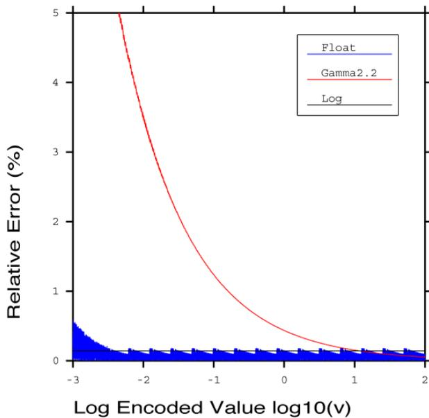
**Figure 5: The relative error is plotted against the log<sub>10</sub> of luminance values for three encoding methods [8].**
