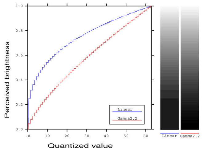
Figure 4: This image shows the perceived brightness using gamma and linear encoding [8]. A 6-bit resolution was used here to make the quantization steps more visible.
