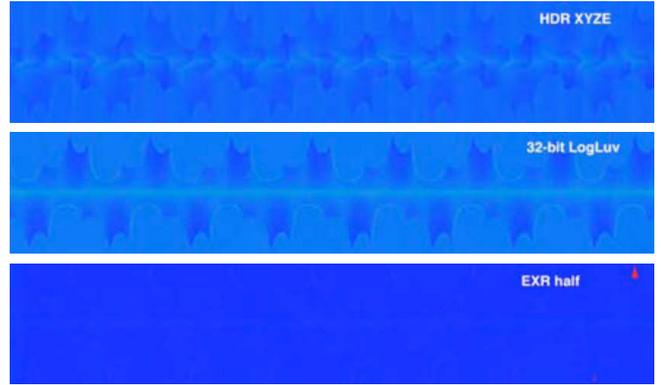
Figure 20: The XYZE, the 32-bit LogLuv and the OpenEXR encoding keep errors mostly under the visible threshold over the entire dynamic range. Only the OpenEXR encoding shows some difficulties in representing a few high saturated colors at high luminance values.
