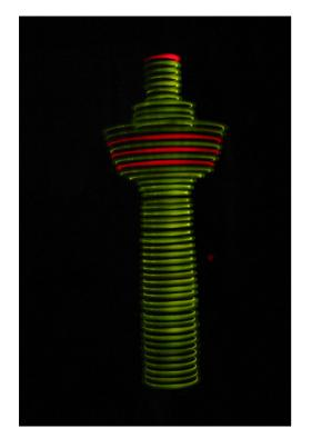
Figure 16: A volumetric display made of rotating leds
