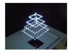
Figure 17: A volumetric display using a pulsed laser to create balls of plasma in air.
