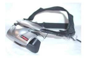
Figure 8: Picture of a modern HMD using LCD's
