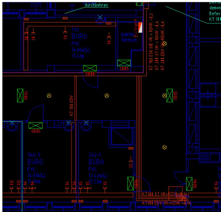
Figure 7: In the background, blue, a floor plan with utilization information for each room is shown. In the middle layer lights for escape routes in green, and annotations in cyan can be seen. The power outlets, cable conduits and annotations in the red foreground make the supply structure easily perceivable.
