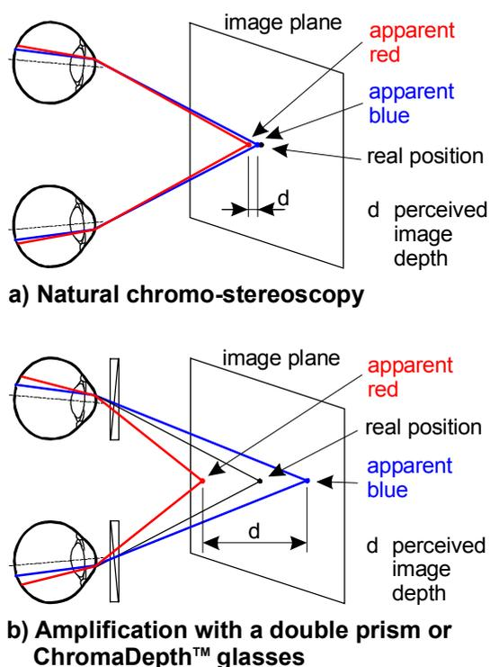
**Figure 1: Principle of chromo-stereoscopy without and with amplification**
