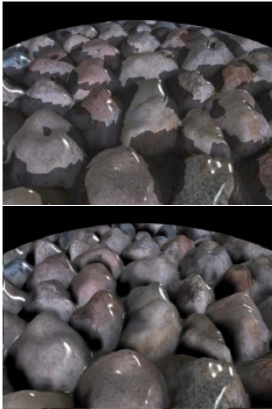
Figure 15: Top: the hard shadows produced by relief mapping, bottom: soft shadows in parallax occlusion mapping. The self occlusion in both images would not be achievable with parallax mapping. [Tatarchuk 2006].
