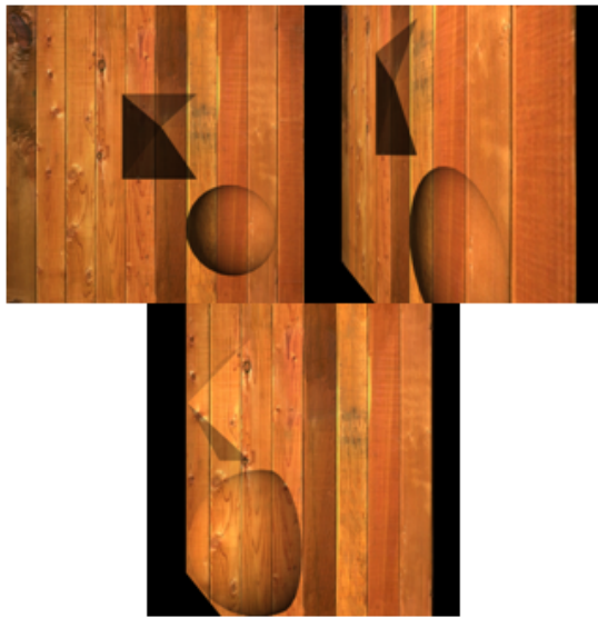
Figure 4: A pyramid and a sphere painted onto a surface using a bump map, top left: viewed from top this somewhat works, top right: from the side the flat nature of the texture is unveiled, bottom: how the image should look, rendered using actual geometry.
