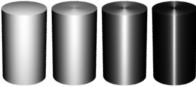
Figure 8: Schlick model: A continuum between isotropic and anisotropic reflection. r = 1.0 , p = \{1.0, 0.5, 0.2, 0.05\} . [Schlick 1994]
