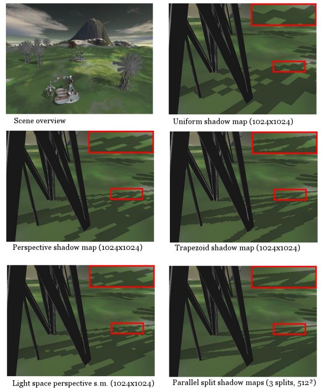
Figure 16: Six shadow map algorithms compared. Images courtesy of Zhang et al.
