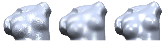
Figure 6: Comparison of different splatting methods. Left: unfiltered splats. Middle: Gaussian weighted splats. Right: Phong Splatting.
