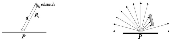
Figure 2: Ray intersecting with obstacle (left) and evenly distributed rays emitted from point P (right)
