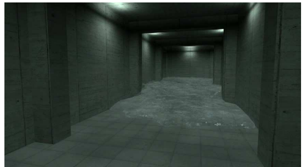
Figure 7: MPS-MAFL simulation of a corridor getting flooded using 100,000 fluid particles. The simulation time is about 3 minutes per frame. (image: [Premzoe 2003])
