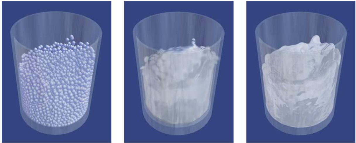
Figure 10: Three different rendering modes: the particles, the surface using point splatting and the iso-surface triangulated via marching cubes. (image: [Müller et al. 2003])
