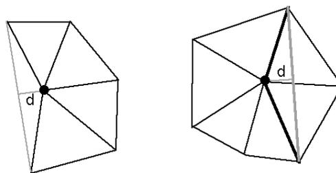
Figure 2: distance measure for boundary vertices (left side) and interior vertices (right side).
