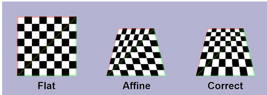
Figure 18: Affine texture mapping does not take into account the depth information of a polygon’s vertices. If a polygon is not perpendicular to the viewer it produces a noticeable defect.
