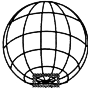
Figure 19: Very fine structures at the pole of the sphere will yield artifacts.
