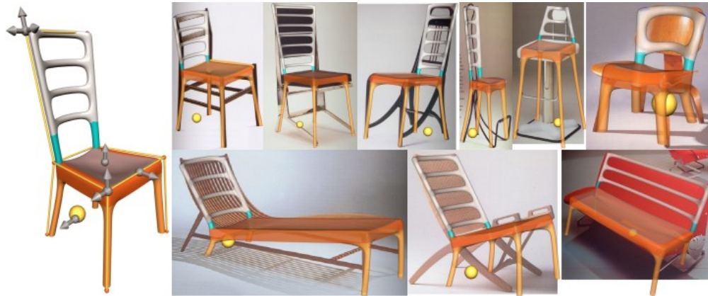
Figure 11: Model of a chair. Changing the parameters of the chair leads to different representations. Images by Sven Havemann 3 [2].
